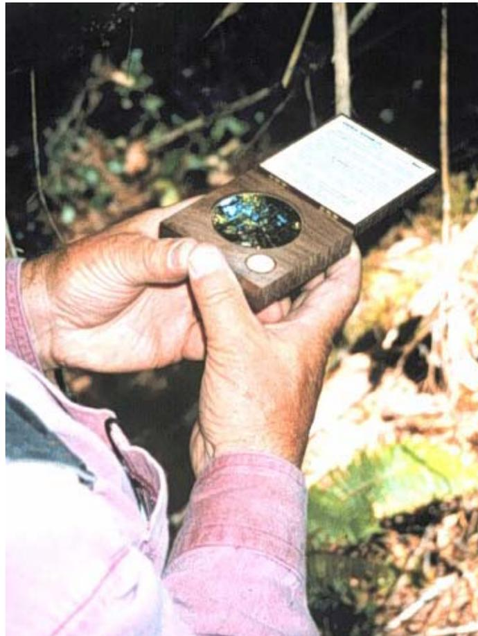
Figure 18. Measuring canopy cover with the spherical densiometer in western Mendocino County in 1996.
