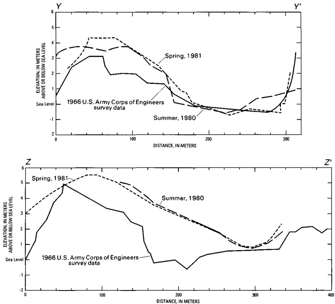
FIGURE 7.—Topographic profiles Y-Y' and Z-Z' across the mouth of Redwood Creek. Profile locations are shown in figure 2.
