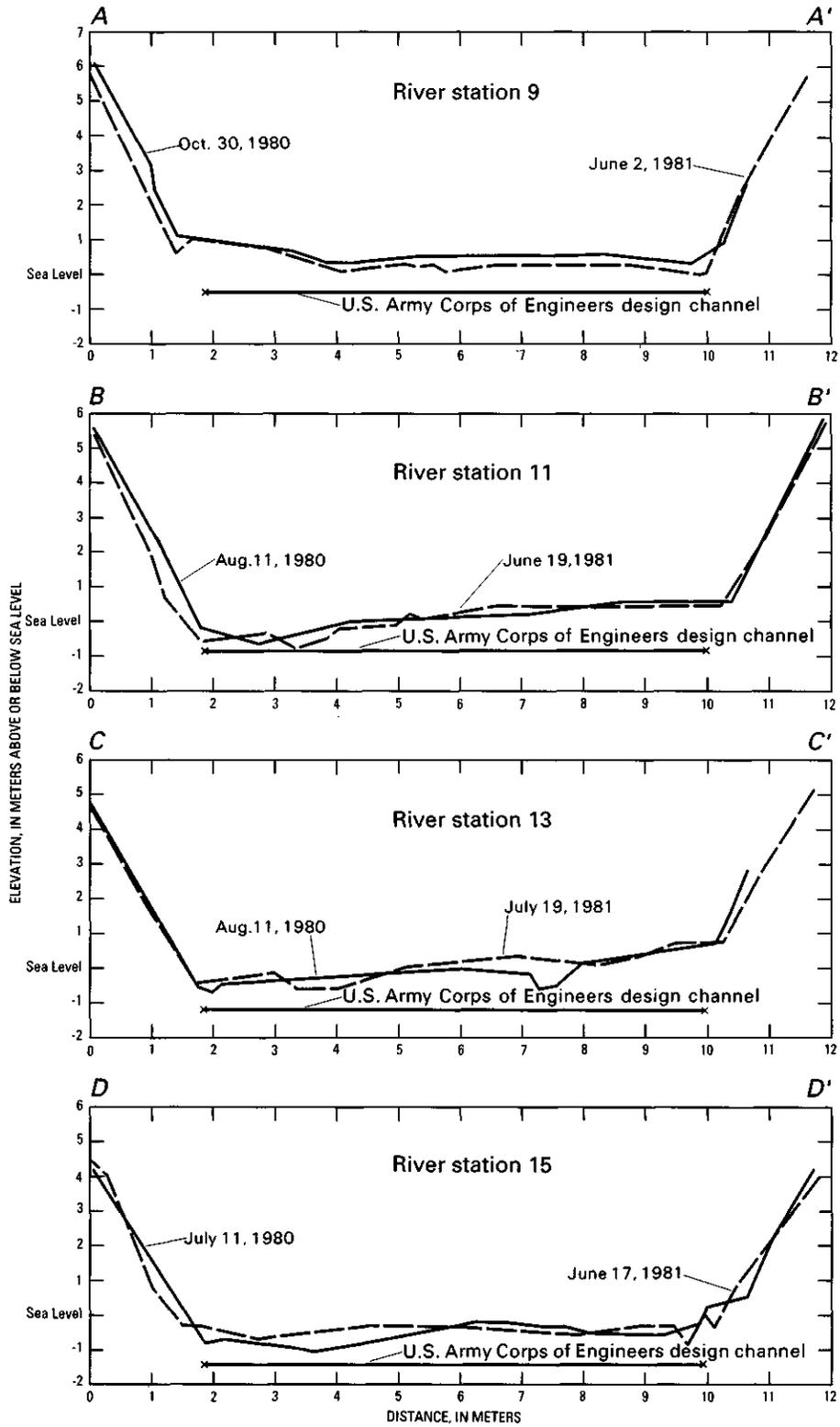
FIGURE 9.—River profiles A-A', B-B', C-C', and D-D' along lower Redwood Creek. River station locations are shown in figure 2.
