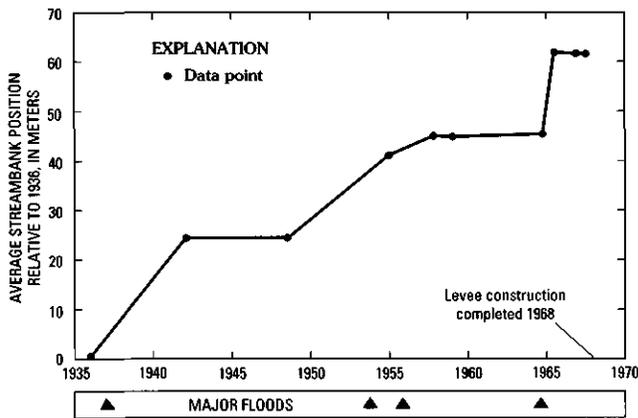
FIGURE 6.—Cumulative southward migration of the last downstream meander at the mouth of Redwood Creek, based on average erosion for the five cross-section lines shown in figure 5. Major floods have peak discharges of at least 1,065 m<sup>3</sup>/s.
